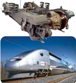
Bogie double-deck TGV motor unit.
