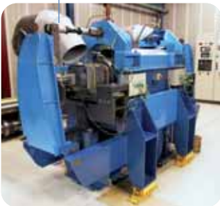
SNR bearing test bench.
